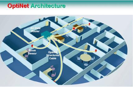
Figure 51: OptiNet Architecture (from Aircuity website)
